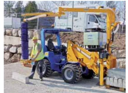
... the vacuum laying machine: Safe, quick and efficient - Jumbo BV-vario.
